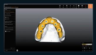
Based on the digitally merged patient data (e.g. DICOM data, intraoral scans, set-up), the dentist can determine the ideal implant positions according to functional and aesthetic aspects, taking bone density into account. Based on such data, the dental technician can produce surgical guides, individual impression trays, models, restorations for immediate loading and resin prototypes.
