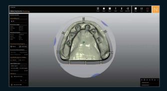
With the CAD/CAM Model Maker software module, the upper and lower master models are designed and then manufactured using a Zirkonzahn milling unit. The models are fitted with laboratory analogues and can then be used to check the final restorations, e.g. resin prototypes with titanium bars.
