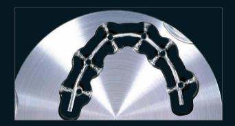
After their elaboration with a Zirkonzahn milling unit, the bars made of high-quality titanium 5 are refined with a surveyor and high-gloss polished. According to one's requirements, the titanium bars can be anodised in a golden shade using the Titanium Spectral-Colouring Anodizer, in order to avoid the grey value shining through the superstructures.
