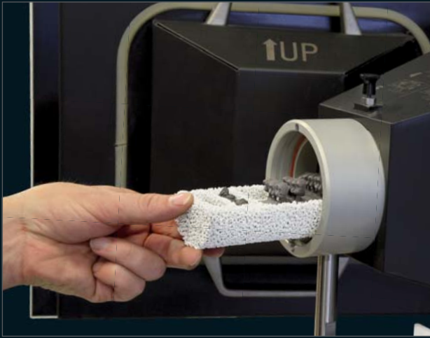
Combustion chamber of the Zirkonofen 700 Ultra-Vakuum sintering furnace for up to 120 zirconia and 25 Sintermetall elements.
