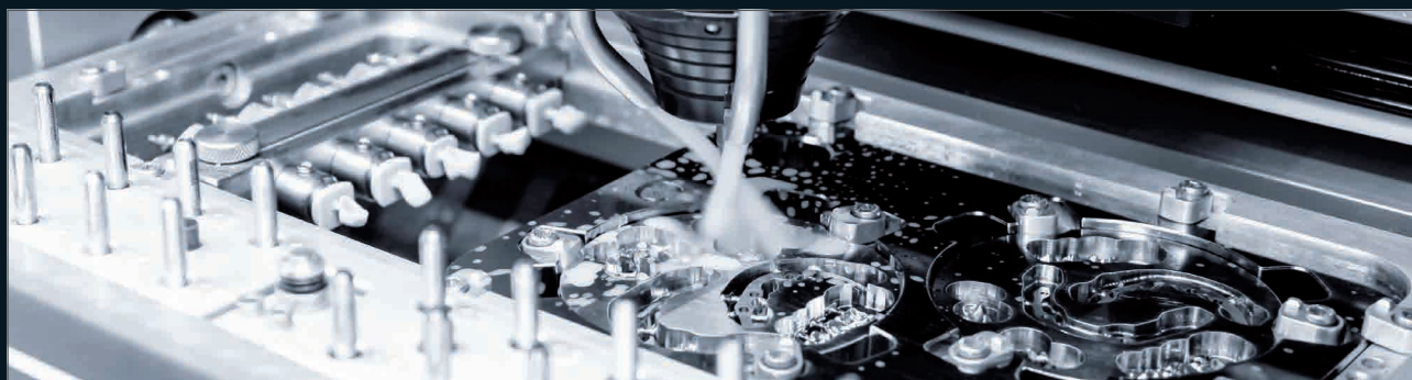
Combination of 2-Blank-Plate and Bridge-Rod Holder M4, Glass Ceramics Holder M4, Combi-Holder Raw/Glass M4 or JawPositioner Support for the elaboration of two material blanks (Ø 95 mm) and 10 Bridge-Rod or glass-ceramic blanks
