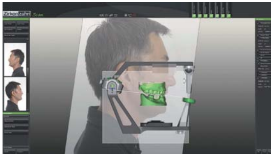
Fig. 1: Ideal situation characterised by a 1:1 transfer of the maxillary position in the skull to the articulator and into the CAD software
