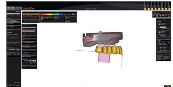
Fig. 22: Positioning of the dental restoration based on the natural occlusal plane
