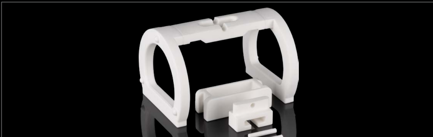
Sintering Holder (ZBAC2188) Suspension device for the sintering of larger Sinternit structures (at least 6 elements) fixed with the Bar Carrier and the Bar Carrier XL in the Zirkonofen 700 Ultra-Vakuum.
