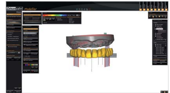
Fig. 23: The position of the absolute midline and of the maxilla are recorded separately using the same reference plane, which permits to reproduce the current situation of the patient in the software
