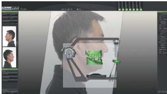
Fig. 1: Ideal situation characterized by a 1:1 transfer of the maxillary position in the skull to the articulator and into the CAD software
