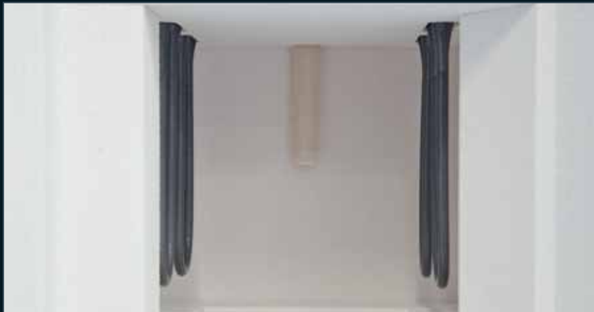
Combustion chamber of the Zirkonofen 700 sintering furnace with MoSi 2 heating elements
