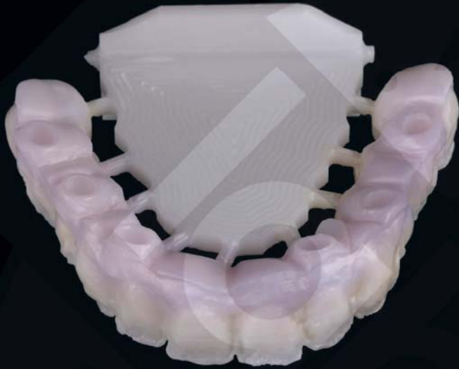
Fig. 17: Coloured and sintered maxillary structure.
