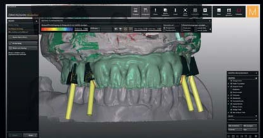
Fig. 16: Maxillary bridge with exit points of the occlusal screw retention.
